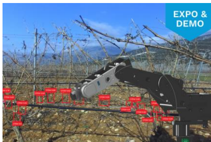
Robotic pruning arm - Robotic Perception
